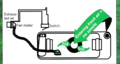
The ventilator is switched on as soon as the blade valve starts to operand is switched off again when the blade valve is closed.
