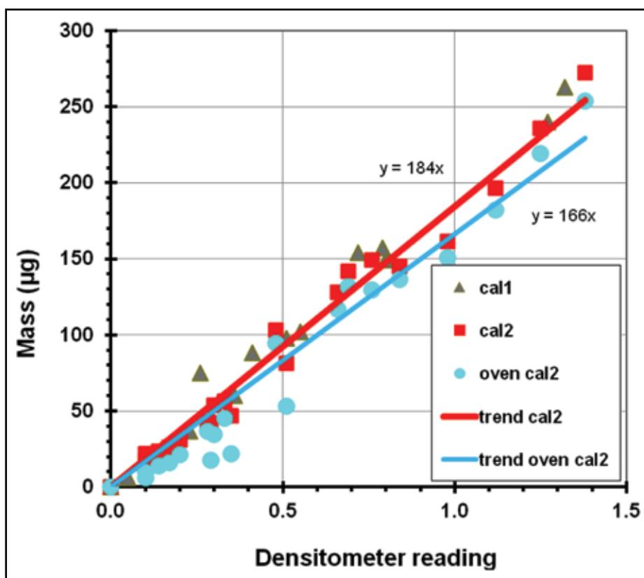
Figure 3. Calibration filter masses compared to densitometer readings show the influence of organic material on the filter masses. Filter weighings are two years apart (cal1, cal2) and after oven-drying (oven cal2). Trend lines are constrained to pass through zero in this and all other plots in this paper.
