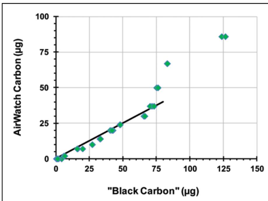
Figure 5. AirWatch grey scale results vs results from the 'smoke stain' M43D reflectometer. Filled diamonds are AirWatch 'cal2' values determined by a panel and reduced by 10% to account for organics. The trend line is for AirWatch concentrations less than 50 µg.
