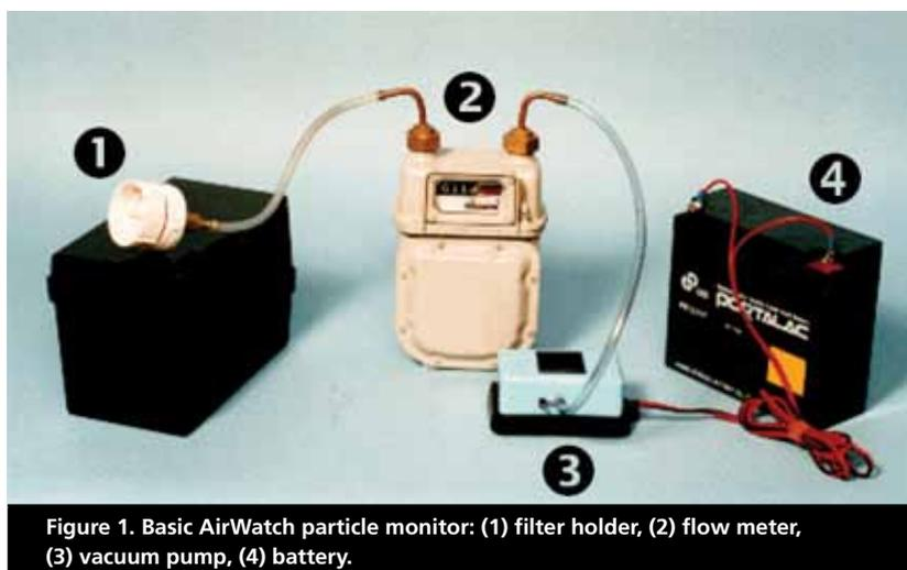
Figure 1. Basic AirWatch particle monitor: (1) filter holder, (2) flow meter, (3) vacuum pump, (4) battery.
