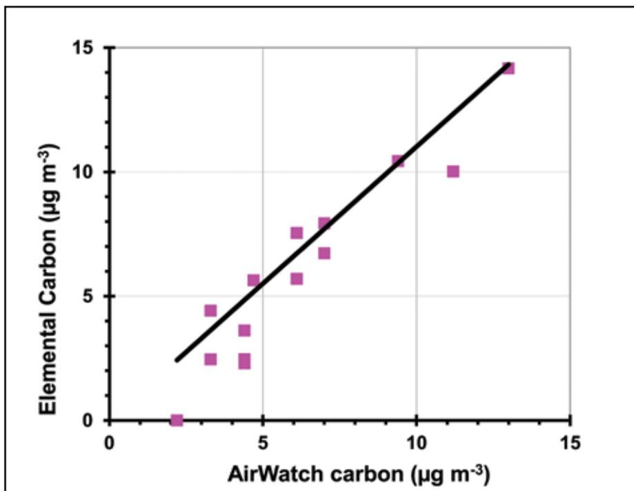
Figure 6. PM<sub>2.5</sub> Elemental Carbon as determined by ANSTO compared with AirWatch particle concentration estimates on the 15 days during the AFP Study (Ayers *et al.* 1999) when AirWatch measurements were also made.
