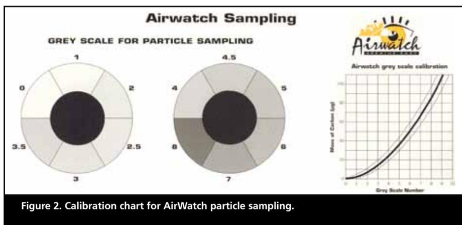
Figure 2. Calibration chart for AirWatch particle sampling.
