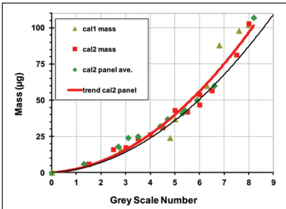
Figure 4. Mass of particles on test filters vs panel selection of segment number from the grey scale calibration chart (Figure 2). 'cal1' and 'cal2' are test filter data obtained two years apart. The black line is the 'cal2 panel' trend line reduced by 10% to account for organics.
