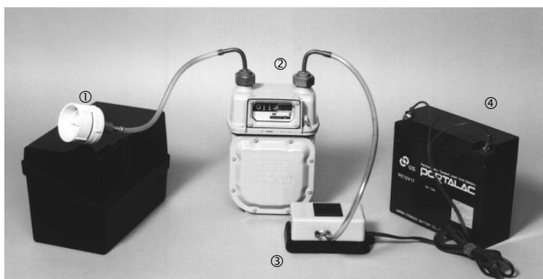
Figure 2. Particle sampling equipment for AIRWATCH
