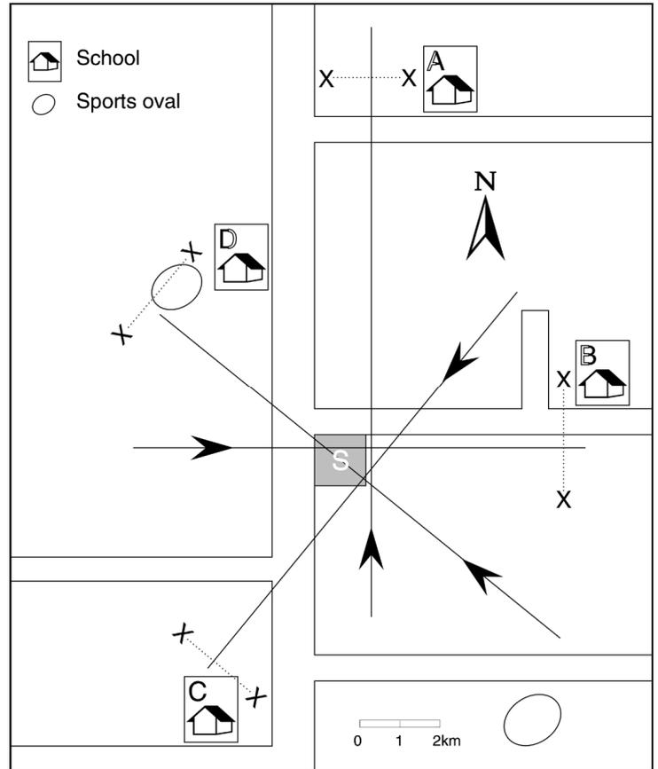
**Figure 5.** Measurements of wind direction when the same odour is smelt under different conditions at locations A, B, C and D allow identification of the source at S.
